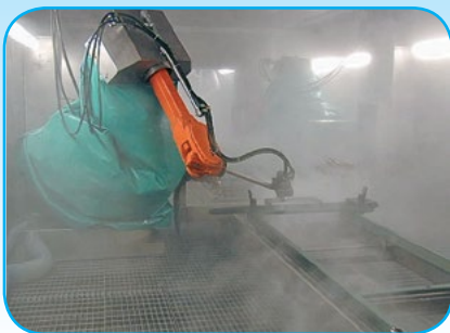
Robotic cleaning of skids at automotive plant 105 lpm/1000 bar
