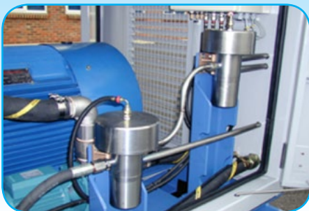
2 valves mounted in series
