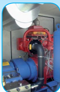
HPS2000 pump driven by a Zone 2 engine
