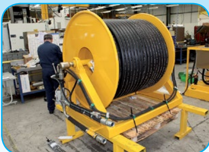
Remote hosereel with 320m of 1 1/2" hose used on a 775lpm at 250bar pump used for large diameter sewer cleaning
