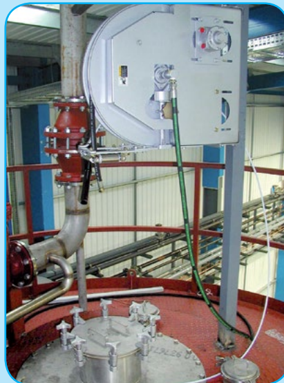
Small air driven reel to lower/raise a tank cleaning nozzle
