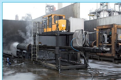
200lpm at 1000bar with a 5 lance bundle blaster
