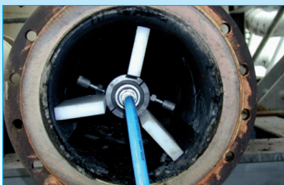
Self-rotating nozzle to give total coverage
