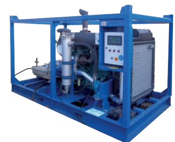
HPS5000DC unit, 200lpm at 1000bar
