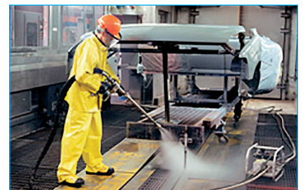
Manual cleaning inside a paint shop, 2500bar
