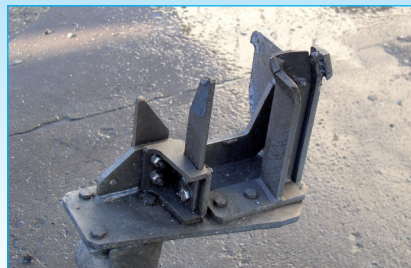
Skid after cleaning at 2500bar at Nissan, UK
