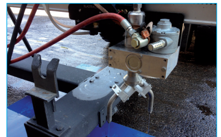
Paint removal from Dolly, 500bar
