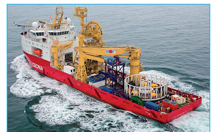
Umbilical & flexible pipe testing equipment aboard the CEONA vessel, Polar Onyx
